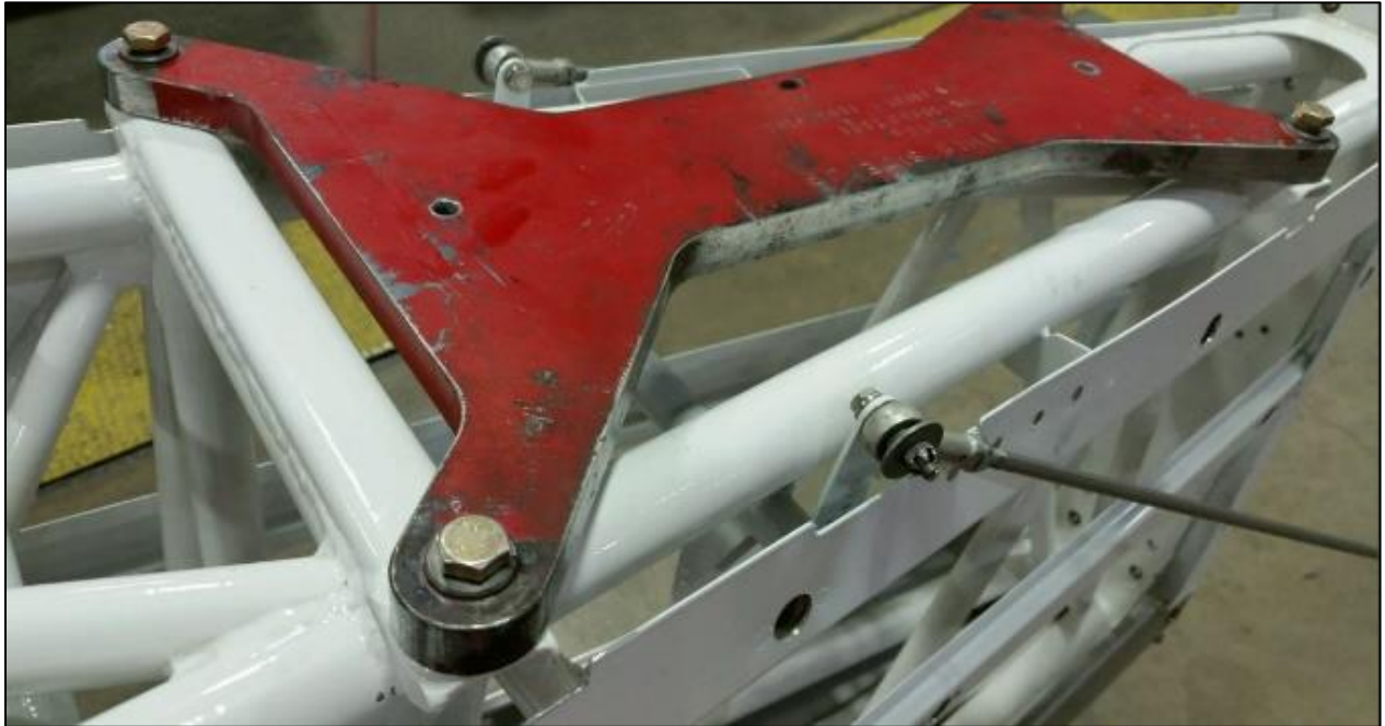
Figure 3. Attach SBAG78-1 Locating Tool to Horizontal Stabilizer in Similar Configuration
